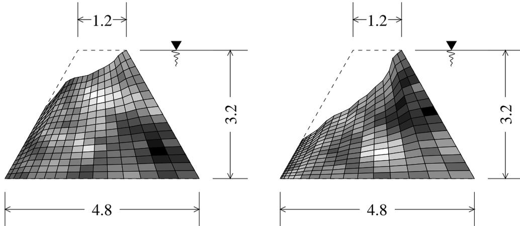
**Figure 1.** FEM discretization of earth dam; two possible realizations.
