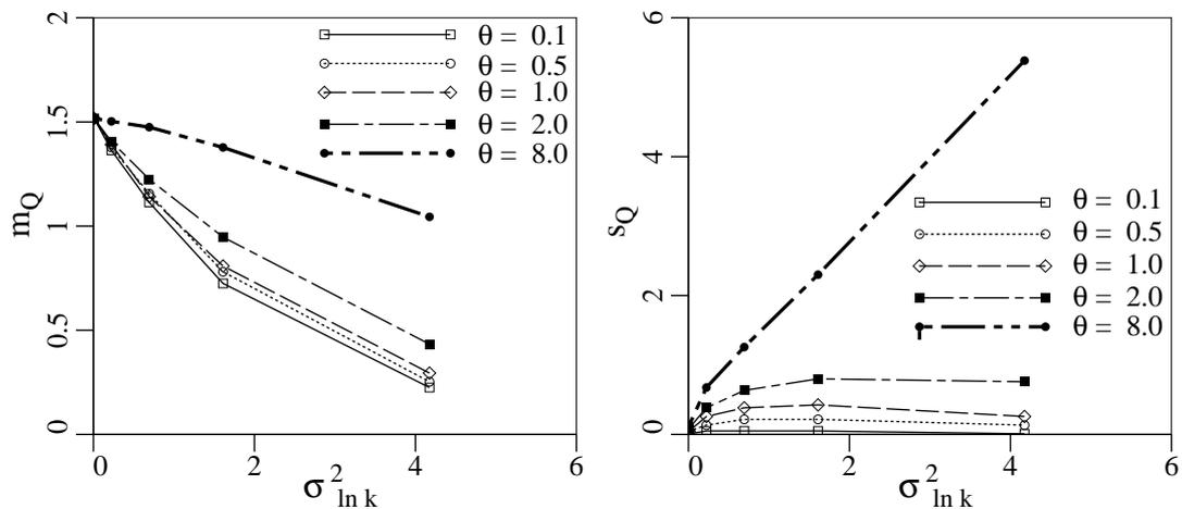
**Figure 2.** Estimated mean and standard deviation of flow rate through the dam.
