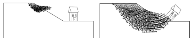
Figure 1. Shallow and deep failure mechanisms in a stratified soil. Both cases have failed, but the consequences are clearly different.
