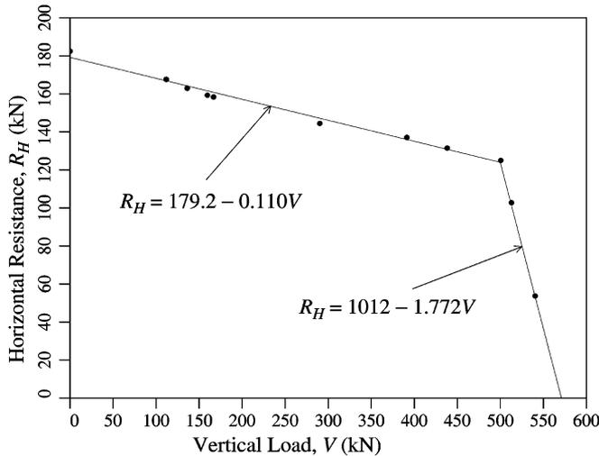
Fig. 3.  $R_H - V$  resistance curve of the tower.
