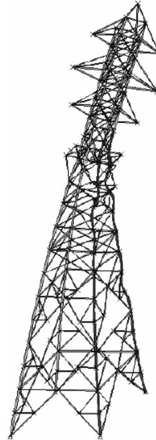
Fig. 2. Tower collapse mechanism.
