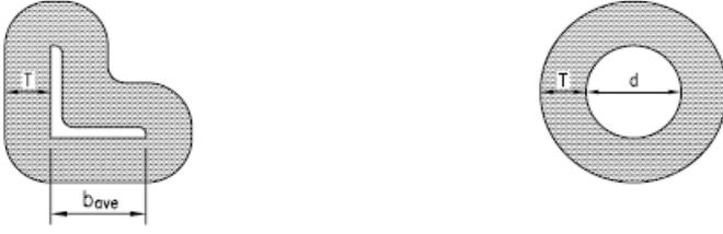
Fig. 5. Ice accretion—typical tower member on left and conductor on right.
