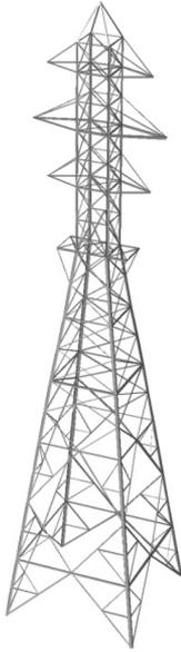
Fig. 1. Double circuit standard suspension tower.
