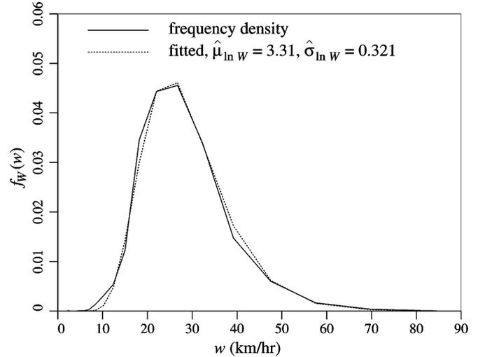
Fig. 4. Frequency-density plot of daily maximum 2-min average windspeed at Halifax airport with superimposed lognormal fit.
