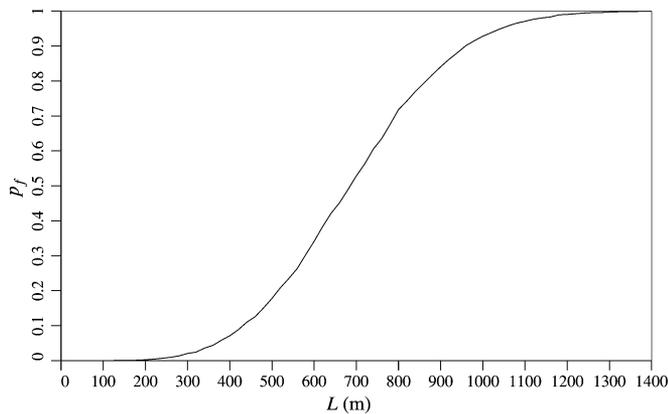
Fig. 7. Lifetime system failure probability versus span length.
