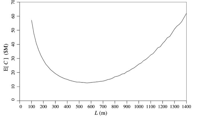
Fig. 6. Expected total lifetime cost versus span length.
