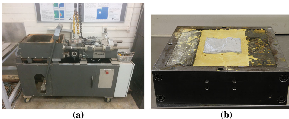
Fig. 14 a View of the Pro Lab shear machine load capacity of 100 kN. b View of the low part of a rock joint specimen encased in one of the steel boxes with plaster
