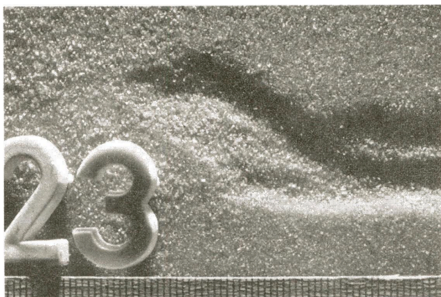
Fig. 3. Photograph of a BEP erosion channel for test number 23 (Hanses, 1985).
